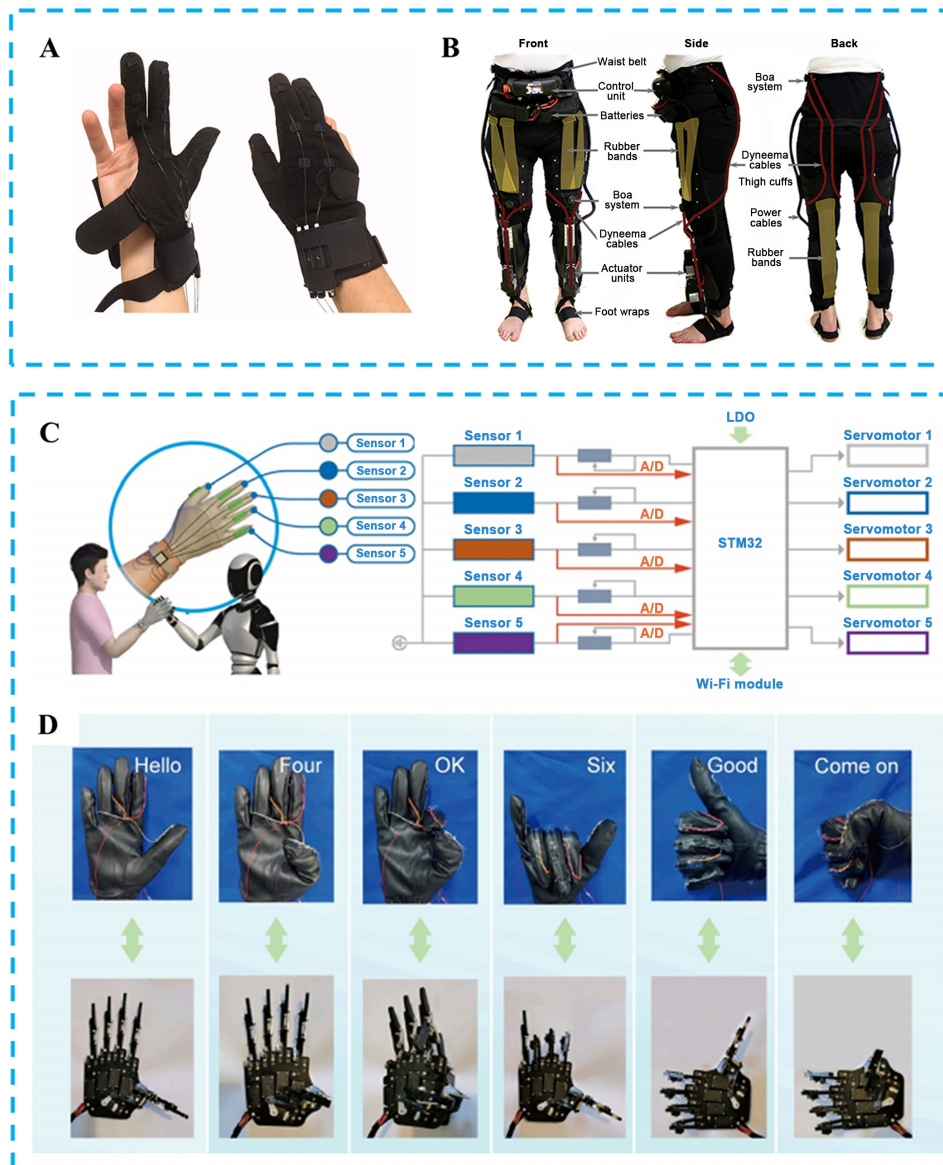
Figure 6. The application of soft wearable robotics. (A) Soft robotic glove for grasping assistance [79] . Reprinted with permission. Copyright 2017, SAGE; (B) The Myosuit for supporting the user's knee and hip joints. Reprinted with permission. Copyright 2017, Frontiers Media [80] ; (C) Schematic diagrams of the smart glove and its controlling circuits and (D) various hand gestures of smart gloves in real-time [50] . Reprinted with permission. Copyright 2017, Elsevier.
